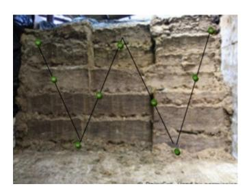
Samples should be taken in the form of a W across the face of the pit (as per example in photograph above).
